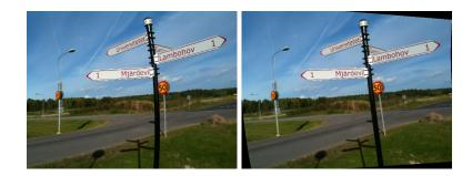
Figure 1: Image acquired during camera rotation on a rolling shutter cell-phone. Left: Video frame from iPhone3GS. Right: Rectification from our CVPR10 algorithm.
